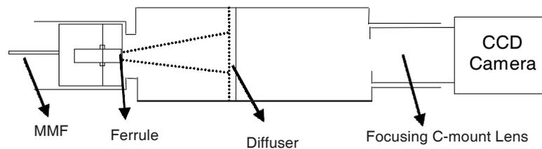
**Figure 3: Schematic Diagram of Sensor Device**
