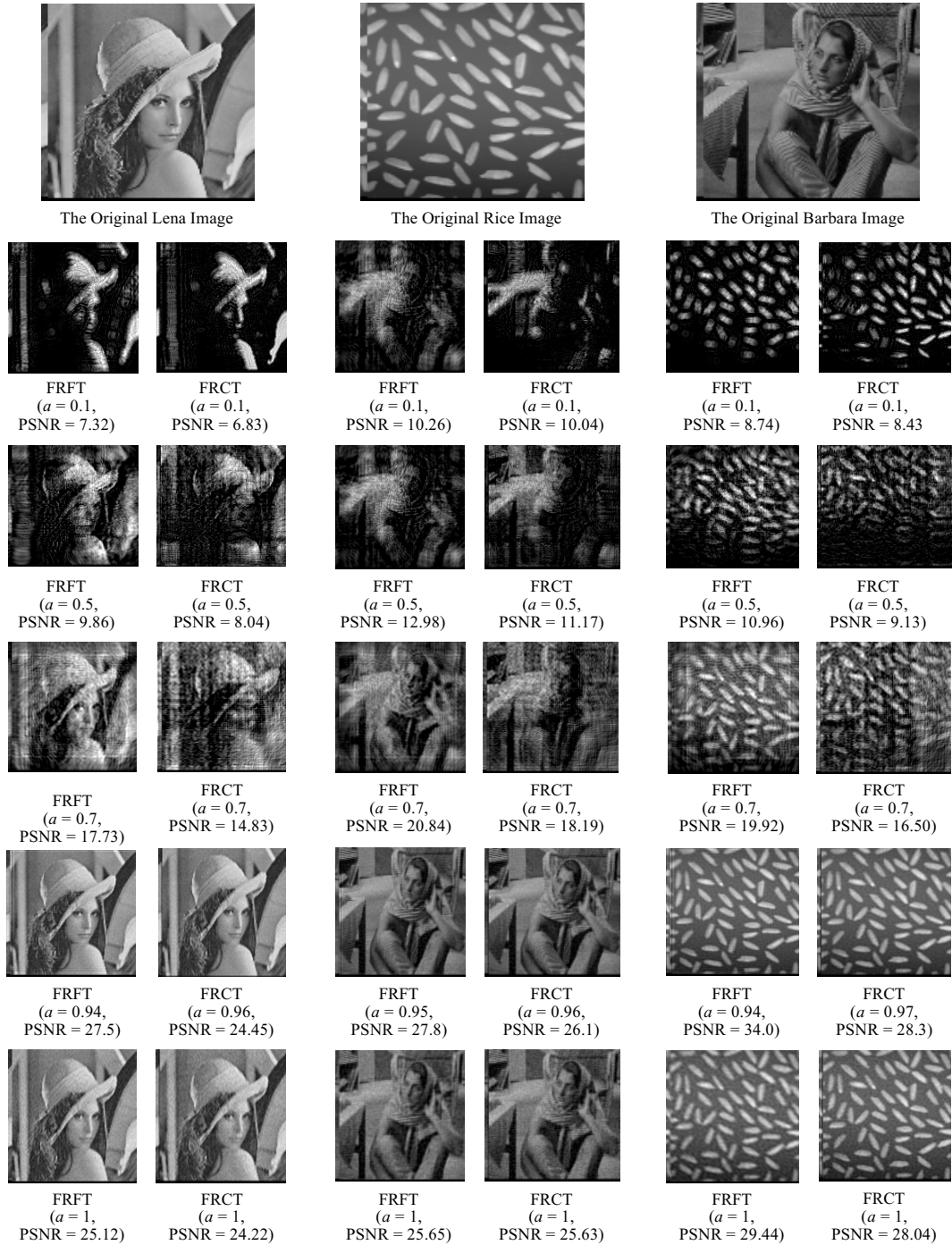
Figure 2: Simulation Results of the Different Images with 256 \times 256 Pixels with CR = 25 for Varying ' a '
