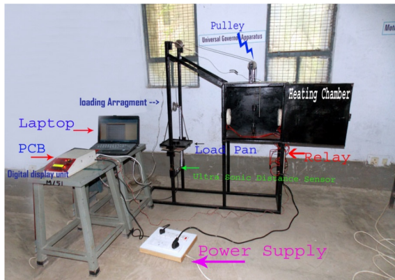
Figure 1: Set up Developed for Creep Testing
