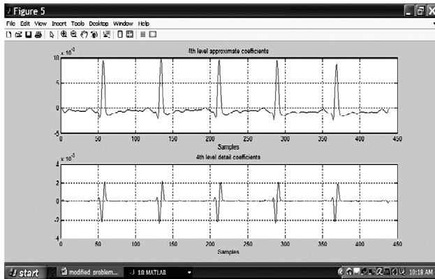
Figure 6: Detected ECG by HAAR, DB1, SYM1, BIOR1.1, RBIO1.1
