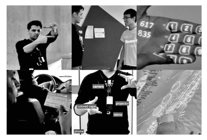
Mobile Component: The Sixth Sense device consists of a web enabled smart phone which process the data send by the camera. The smart phone searches the web and interprets the hand gestures with help of the coloured markers placed at the finger tips.
