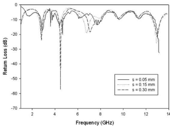
Fig. 2: Simulated  $|S_{11}|$  Performance of Proposed Varying Scale-Factor Monopole Structure with Change in Ring Widths
