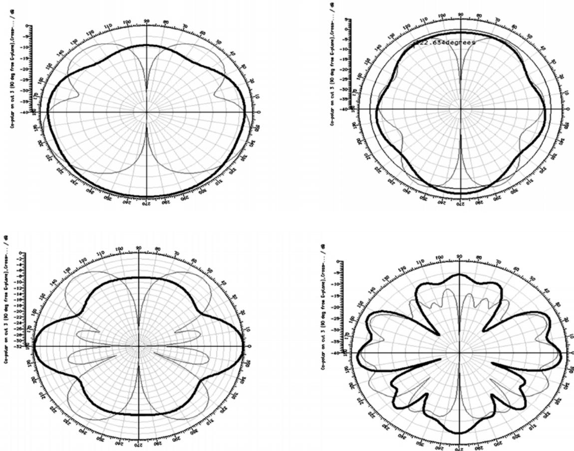
**Fig. 5:** Radiation Pattern of the Sierpinski Monopole Antenna 90° From E-Plane
