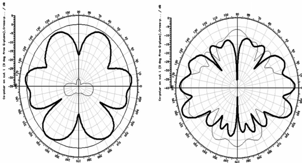
**Fig.4:** Radiation Pattern of the Sierpinski Monopole Antenna 0° From E-Plane
