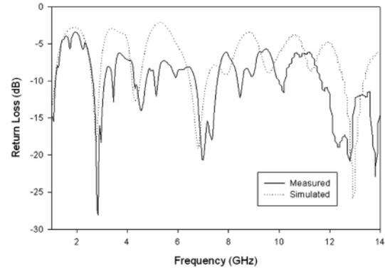
Fig. 3 : Measured  $|S_{11}|$  Performance of Proposed Varying Scale-Factor Monopole Structure.
