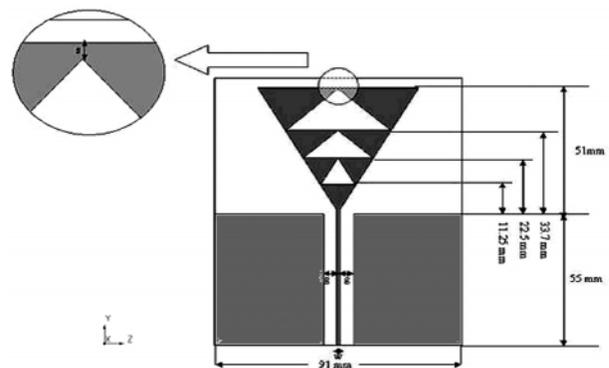
**Fig. 1:** Geometry of Proposed CPW-fed Third Iteration Sierpinski Monopole with Varying Scale Factor  $\delta = 1.5, 1.5, 2$  and Flare Angle  $\alpha = 60$  (total size 106 \* 91 mm<sup>2</sup>).
