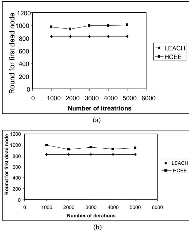
**Figure 3:** Round for Death of First Node using (a) LEACH ( $m=0, \alpha=0, \beta=0$ ) and HCEE ( $m=0.1, \alpha=1, \beta=0$ ) (b) LEACH ( $m=0, \alpha=0, \beta=0$ ) and HCEE ( $m=0.1, \alpha=1, \beta=1$ )
