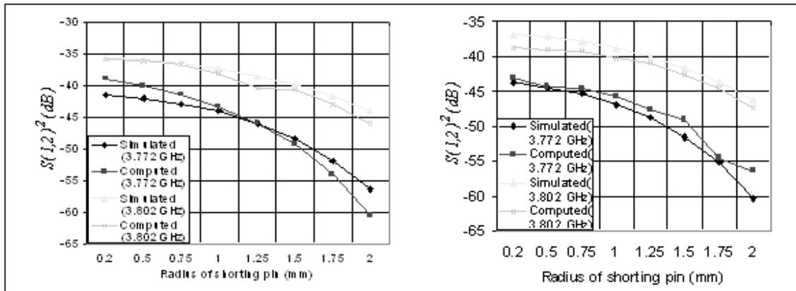
**Figure 3:** Variation of Mutual Coupling Parameter  $S(1, 2)$  with Radius of Shorting Post for (a) Gap between Adjacent Edges = 0.5 mm, and (b) Gap between Adjacent Edges = 1 mm
