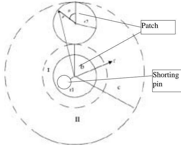
**Figure 1:** Two Gap Coupled Circular Patch Antennas Loaded with Shorting Post.
