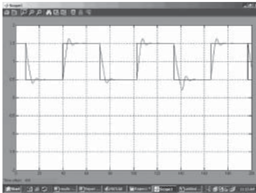
Figure 8: Response of Liquid Level Controller using PID Controller
