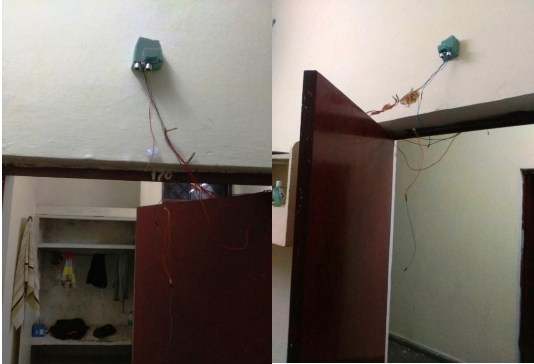
Figure-2: Ultrasonic Sensors deployed on both sides of the room entrance
