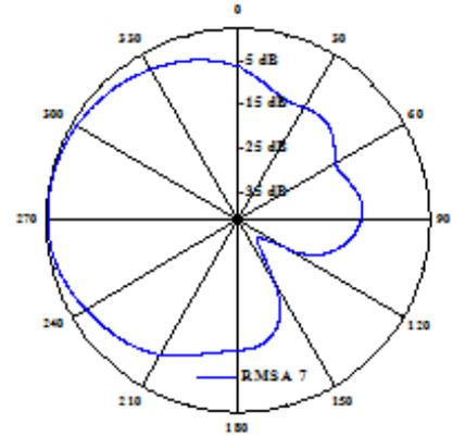
Figure-6 Radiation pattern of SCRMSA(D=0.4 cm)
