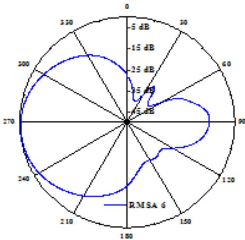
Figure-7 Radiation pattern of SCRMSA(D=0.6 cm)
