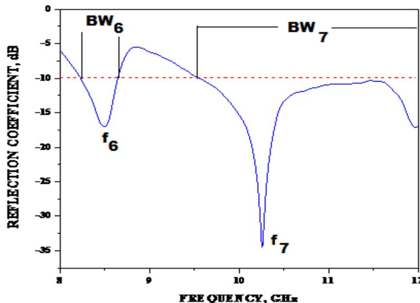
Figure-4 Variation of Return loss versus Frequency of SCRMSA when D=0.6cm
