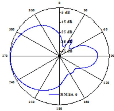
Figure-5 Radiation pattern of SCRMSA(D=0.2 cm)
