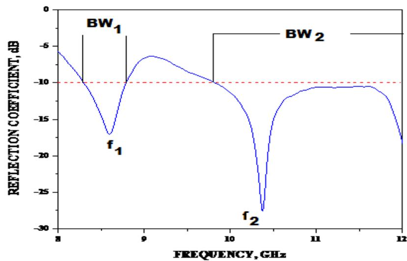
Figure-2 Variation of Return loss versus Frequency of SCRMSA when  $D=0.2\text{cm}$
