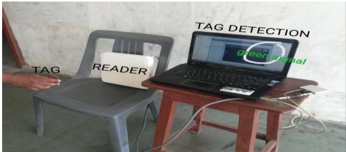
Fig. 10. Set Up for Antenna Testing.
