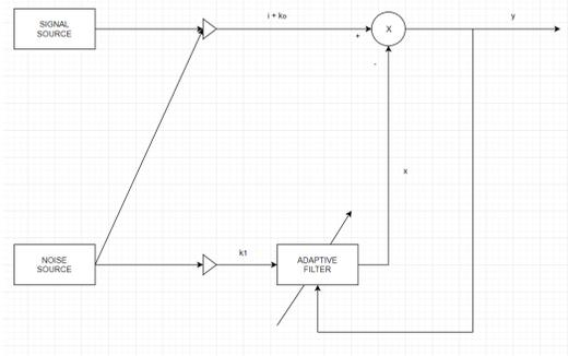
Figure 1. Basic Structure of Adaptive Filter
