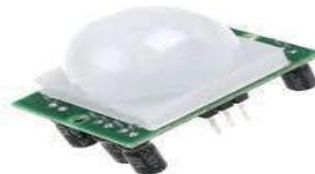
A **passive infrared sensor (PIR sensor)** is an electronic sensor that measures infrared (IR) light radiating from objects in its field of view. They are most often used in PIR-based motion detectors. PIR sensors are commonly used in security alarms and automatic lighting applications. PIR sensors detect general movement, but do not give information on whom or what moved. For that purpose, an active IR sensor is required.
