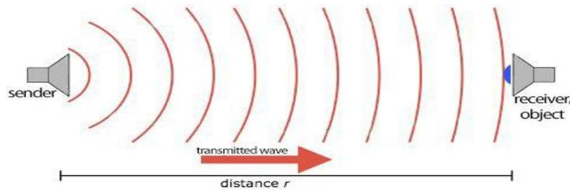
Fig.4a: Direct Measurement Mode
