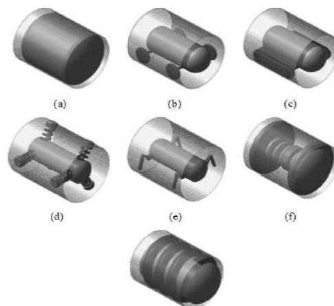
Fig.3: Classification Of In Pipe Robots (A) Pig Type (B) Wheel Type (C) Caterpillar Type (D) Wall Press Type (E) Walking Type (F) Inchworm Type (G) Screw Type[1]
