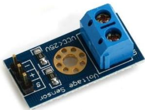
Fig.2.2 Voltage Sensor
