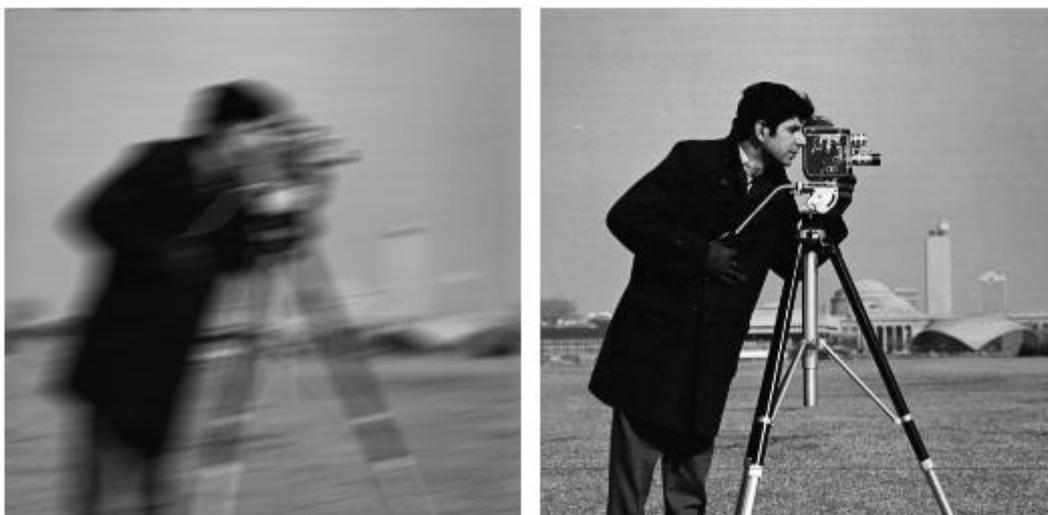
Figure 2.Example of image restoration using Wiener filter
