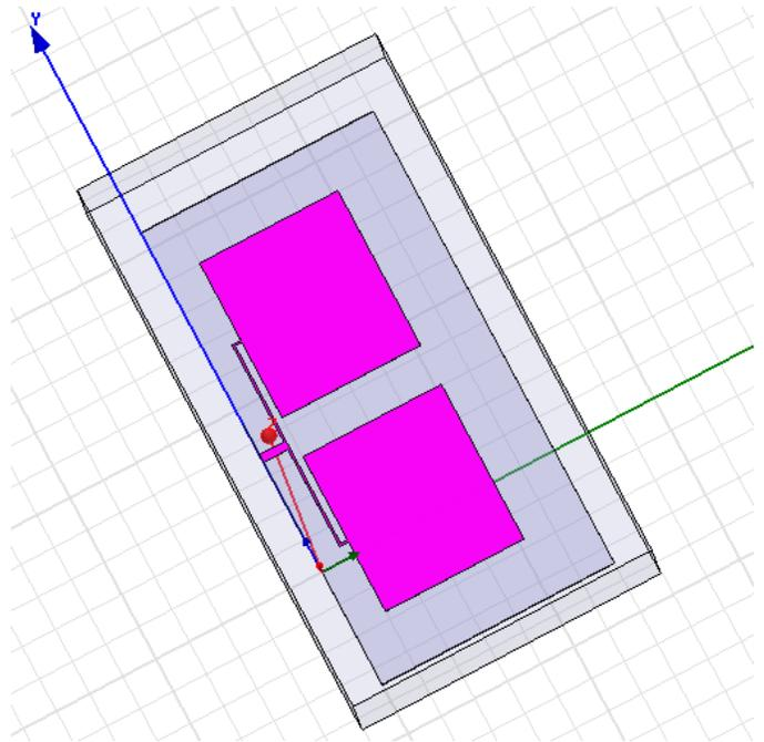
Fig (9) Microstrip patch antenna array using HFSS
