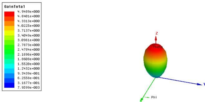
Fig (7) Polar radiation pattern
