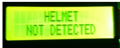
Figure. 4.5 Lcd Display of Helmet Detection
