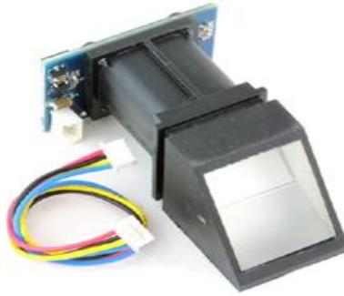
Figure 1: Fingerprint Sensor
