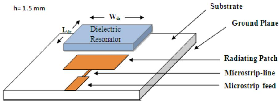
Figure 1. Geometry of rectangular dielectric resonator antenna
