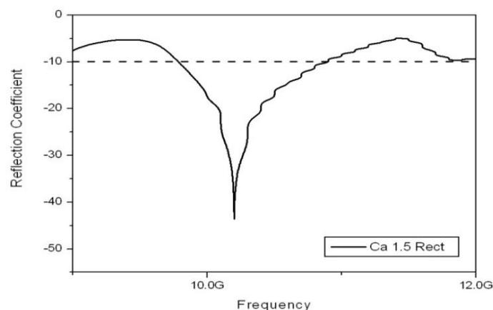
Figure2. Variation of reflection coefficient versus frequency of CaCO<sub>3</sub> Rectangular DRA with thickness h= 1.5 mm
