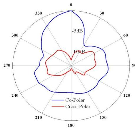
Figure 3. Radiation pattern of proposed antenna at 10.19 GHz
