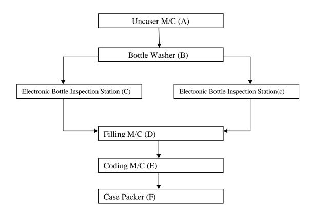
Figure 1. Schematic flow diagram of soft drink Plant
