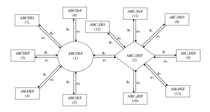
Fig. 4.2: State Transition Diagram of soft drink filling station
