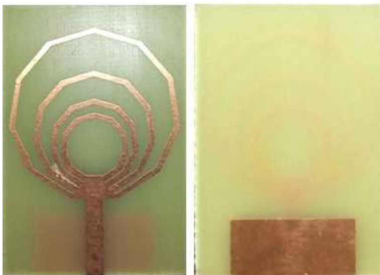
Fig.12. Prototype of Proposed HRF antenna a) Top view b) Bottom view
