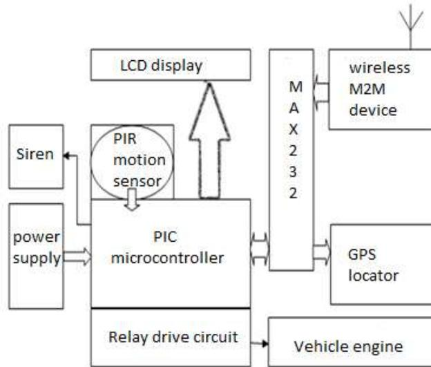
**Fig: functional block diagram of vehicle tracking system**
