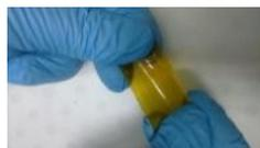
Figure 3. Polyimide substrate peeled-off from Si substrate after CNTTFTs fabrication.
