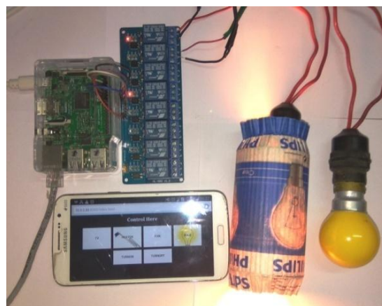
Fig 4: Raspberry Pi interfaced with relay board and appliances
