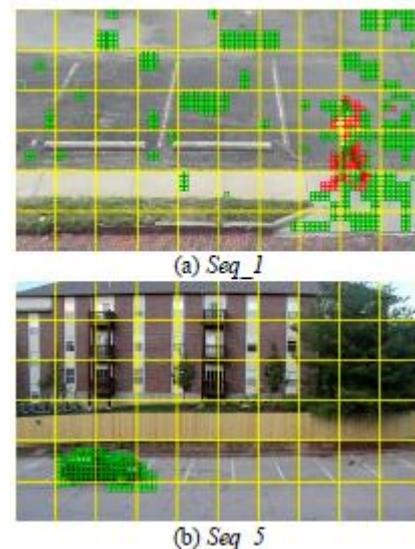
**Figs. 9 The distribution of intra mode within the moving objects (blocks with red borders are encoded with intra mode, blocks with green borders are encoded with inter mode and non-zero MVs, and other blocks are encoded with intermode and zero MVs).**
