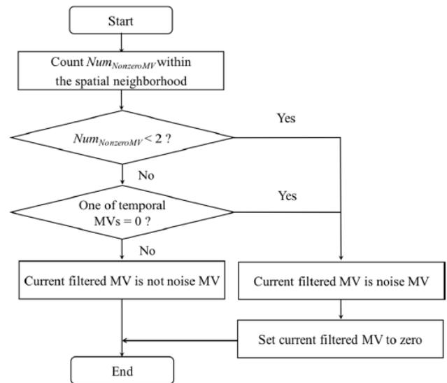
**Fig.4. MV refining for the filtered non-zero MVs.**
