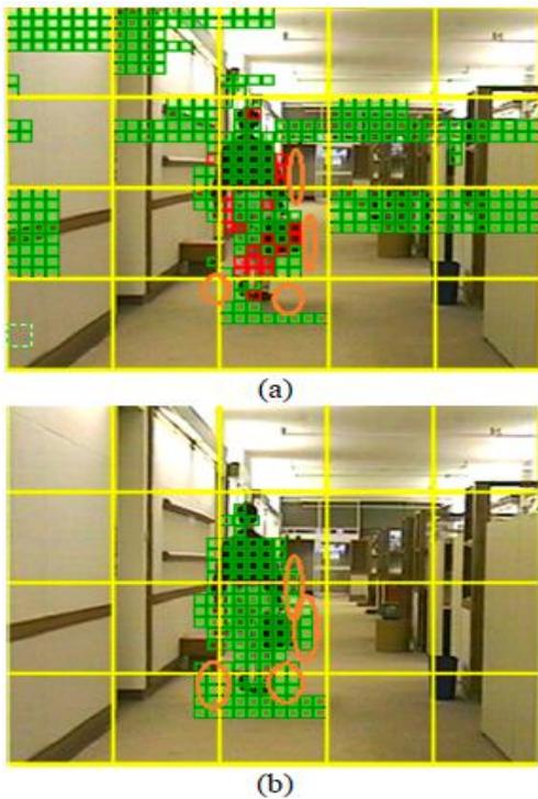
**Figs. 3 (a) an example of original motion vectors; (b) their associated filtered motion vectors.**
