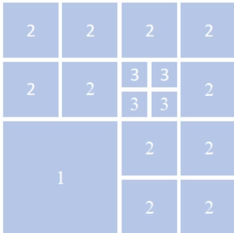
**Fig. 7 The relationship between the depth level and CU size.**
