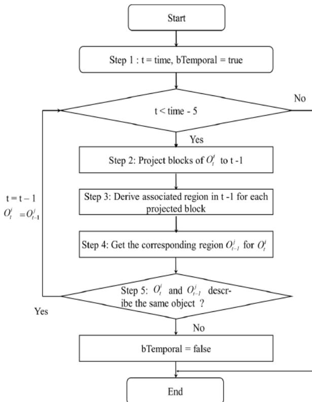
Fig. 5 The flowchart of object region tracking in backward direction.
