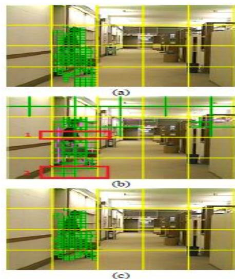
**Figs. 8 (a) Moving object region without boundary refinement; (b) CU and PUsizes of the whole frame; (c) Moving object region after boundary refinement.**
