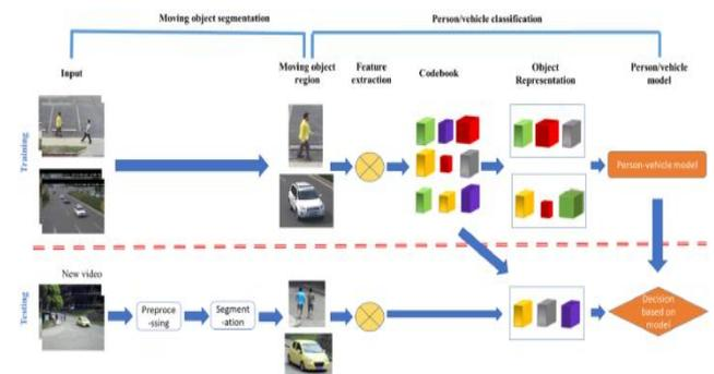
**Fig. 1 The proposed framework for HEVC compressed domain moving object segmentation and classification.**
