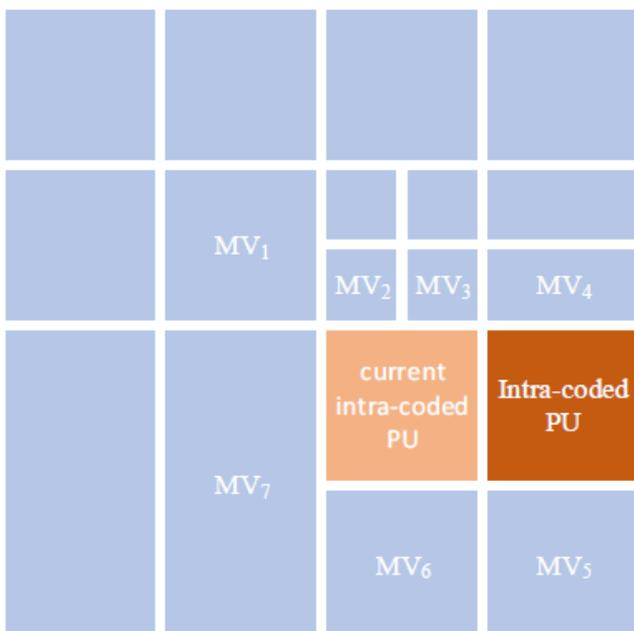
**Fig. 2** MV assignment for an intra-coded PU. One of the first-order neighboring PUs is also intra-coded, and the remaining variably sized neighboring PUs have MVs.
