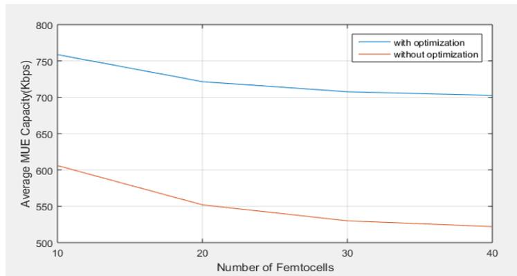
Fig. 1 Average capacity of MUE
