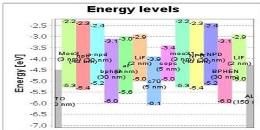
Figure 2. Energy level diagram of various layers used in proposed design
