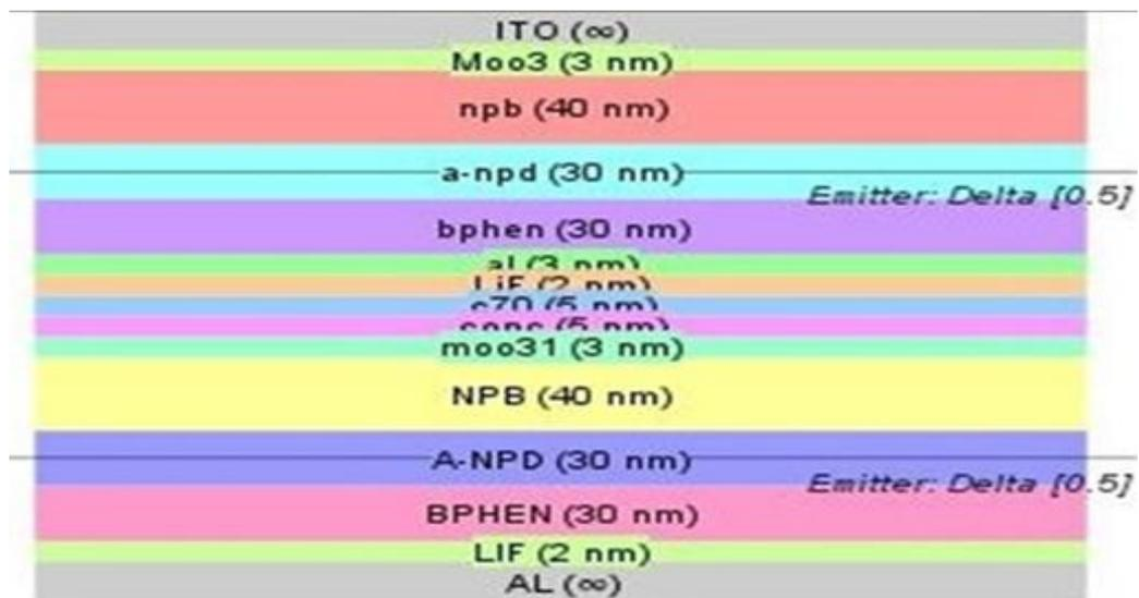
Figure 1. Proposed Device Structure
