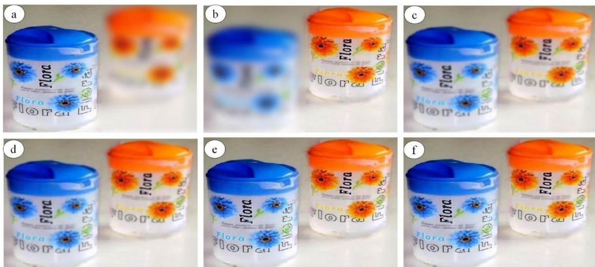
Figure 2: Visual analysis of felora image (a) Partially blurred image 1, (b) Partially blurred image 2, (c) DWT, (d) BWT, (e) NSCT, and (f) Proposed technique
