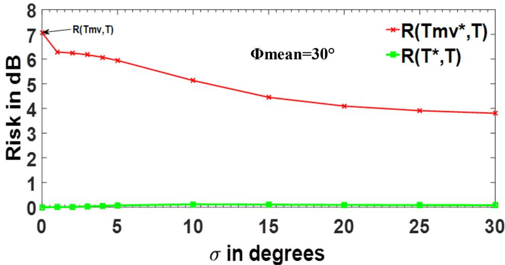
Figure.4. Variation of Risk  $R(T_{mv}^*, T)$  and  $R(T^*, T)$  with dynamic RCS modelled using the Gaussian distribution
