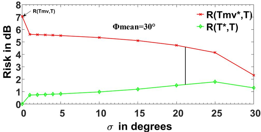
Figure 6. Variation of Risk  $R(Tmv^*, T)$  and  $R(T^*, T)$  with dynamic RCS modelled using the Weibull distribution
