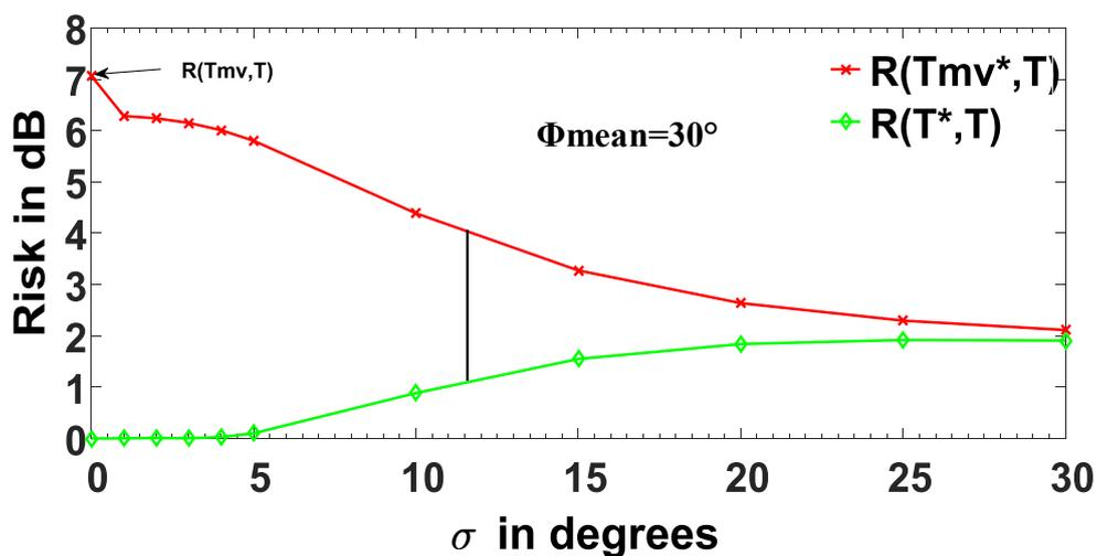
Figure 5. Variation of Risk  $R(T_{mv}^*, T)$  and  $R(T^*, T)$  with dynamic RCS modelled using the lognormal distribution
