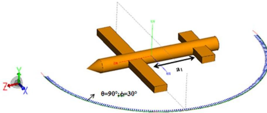
Figure 1. PEC aircraft model and schematic view of directions at which the static RCS are computed
