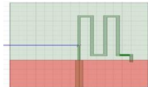
Figure 2b: Bottom view of the proposed antenna geometry
