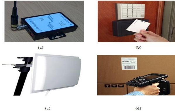
Fig. 1 (a) Active RFID Reader [4] (b) Passive RFID Reader [4] (c) Fixed RFID Reader [4] (d) Mobile RFID Reader [4]
