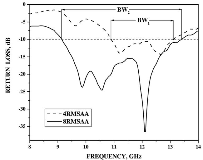
Figure 3: Variation of Return Loss versus Frequency of 4RMSAA and 8RMSAA
