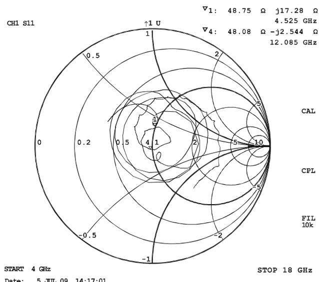
Figure 6: Input Impedance Profile of 8RMSAA
