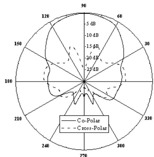
Figure 4: Variation of Relative Power versus Azimuth Angle of 4RMSAA at 12.64 GHz
