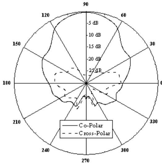
Figure 5: Variation of Relative Power versus Azimuth Angle of 8RMSAA at 12.08 GHz
