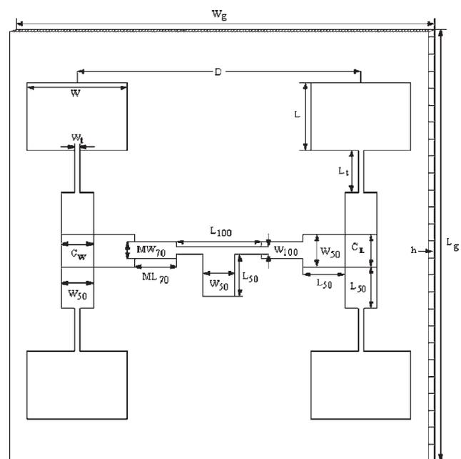
Figure 1: Geometry of 4RMSAA
