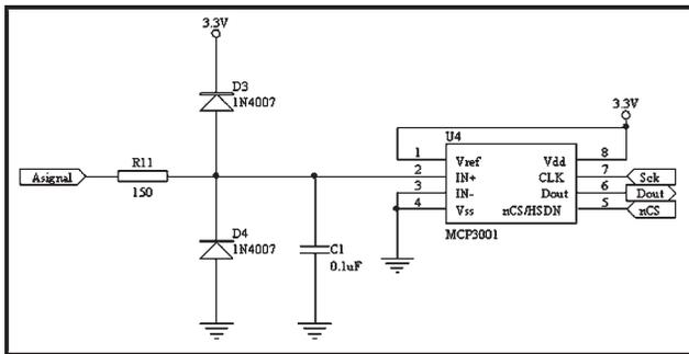
Figure 11: A/D Converter Circuit.
