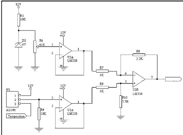
Figure 10: The Circuit of Sensor Node.
