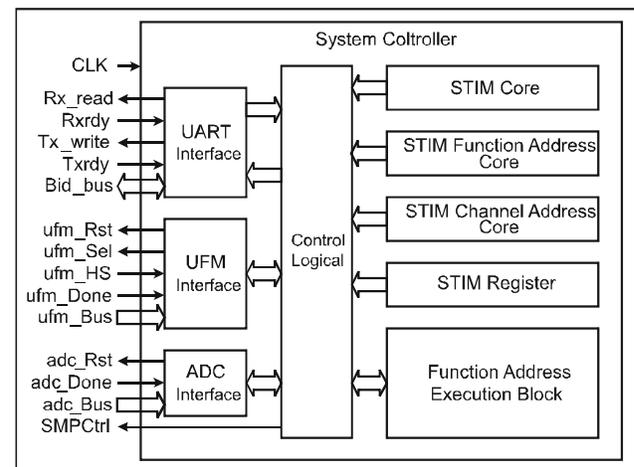
**Figure 6:** Block Diagram of Controller.
