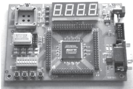
**Figure 16:** Realizing STIM in MAX II CPLD.
