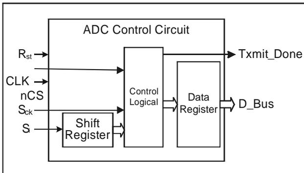
Figure 8: ADC Control Circuit.
