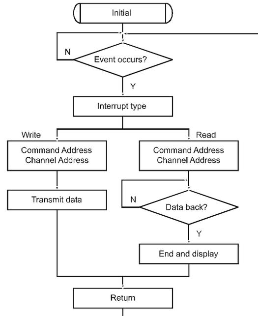
Figure 13: The Control Flow of NCAP
