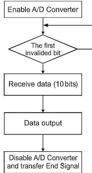
Figure 9: The Signal Conversion Flow of ADC.
