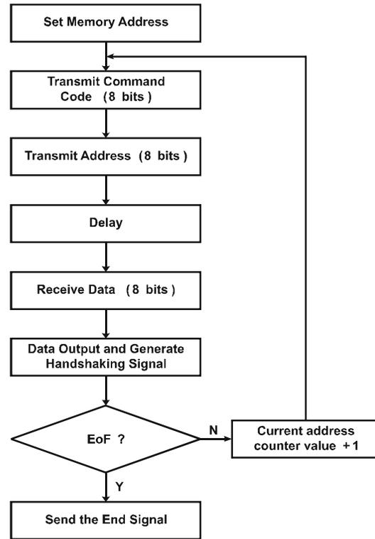
**Figure 5:** The Control Flow in UART.
