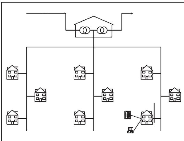
**Figure 1:** Local Area Network of a Distribution Transformer Substation.
