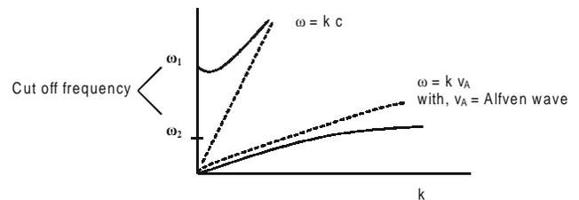
**Figure 5:** Dispersion Relation for a LCP Wave Propagating Parallel to the Magnetic Field in Magnetized Plasma.
