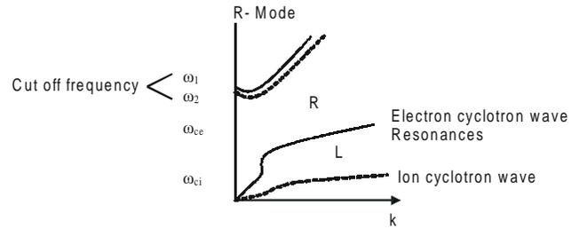
**Figure 4:** Dispersion Relation for RCP Mode of Propagation with  $\omega_{pe} \gg \omega_{ce}$  High Density Limit.
