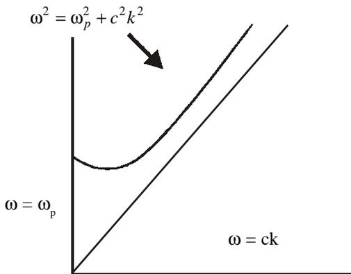
Figure 1: Wave Propagation in Non-magnetized Plasma
