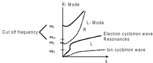
**Figure 3:** Dispersion Relation for RCP Mode of Propagation with  $\omega_{pe} \ll \omega_{ce}$  Low Density Limit.
