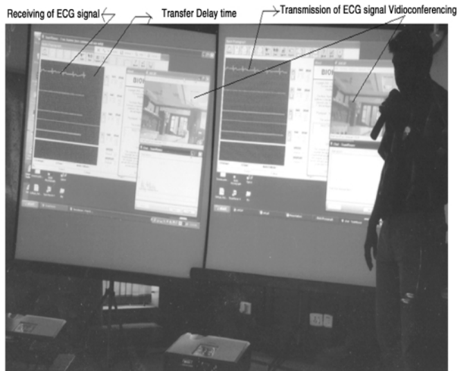
Figure 14: Live Transmission and Receiving of ECG Signal by TM using Computer Communication Network
